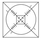
If you know the center point, start with one of the diagonals. You can use a carpenters square to get a general idea of where to put the second diagonal. Then you measure the outside square at 40 feet on each side. Next you can lay the circle and the hash marks as listed above.
