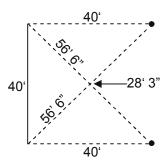
6. With the end and center points marked, you can now lay the tape for the other sides of the square and the diagonals.
