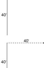
2. From both ends of that line, measure 40 feet at an approximate right angle to the first line, and make temporary marks on the floor.
